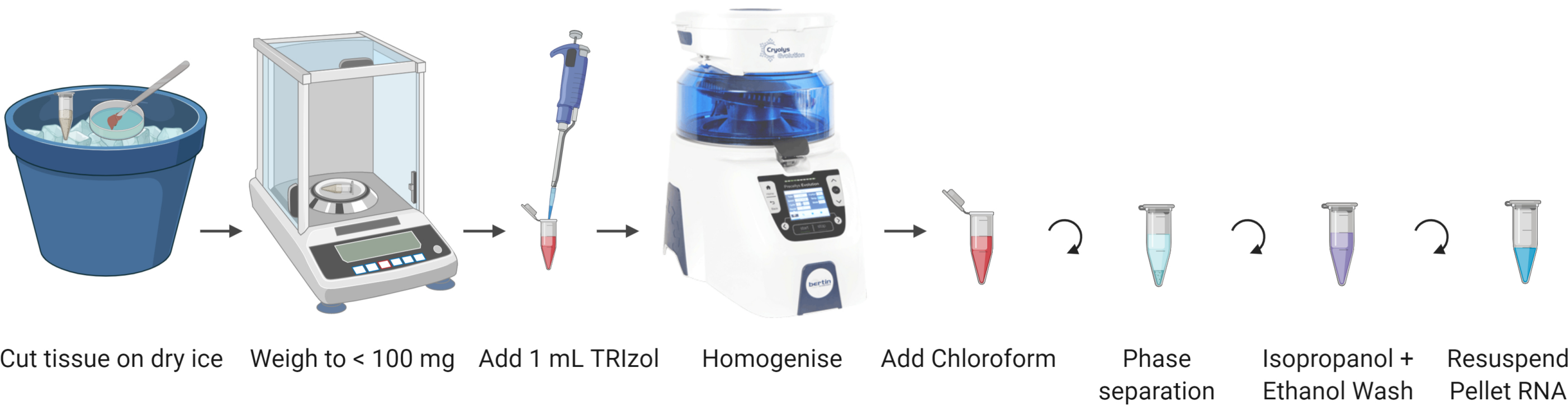
Figure 2a: Workflow for the preparation of purified RNA from tissues.
